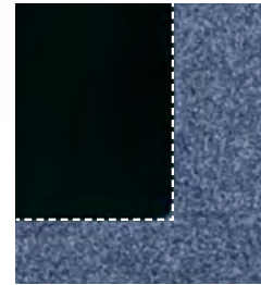
无切削残余的直角 Straight corner with no uncut residue
