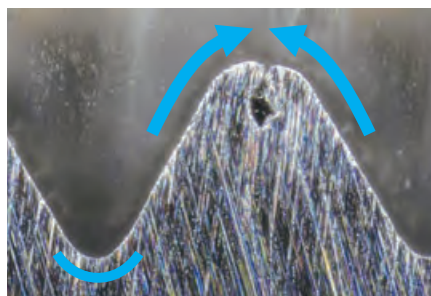
使用GRT加工的内螺纹牙 Internal threads machined by GRT
