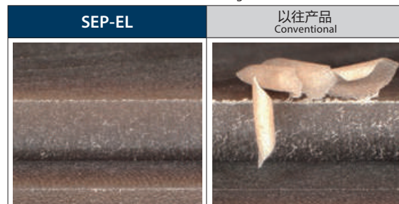
加工60m时的加工面情况 Condition of machined surface after milling 60 m
