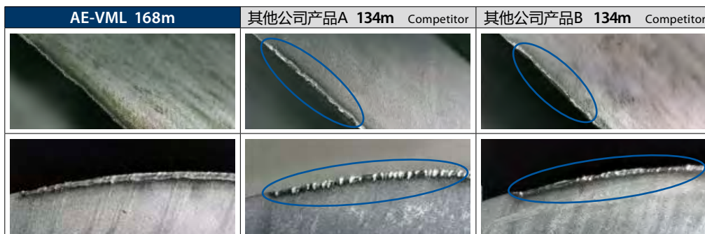
外周刃的磨损状态 Wear comparison of the peripheral cutting edge
