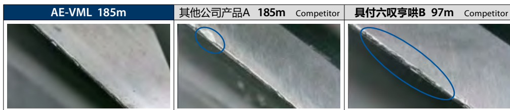
外周刃的磨损状态 Wear comparison of the peripheral cutting edge
