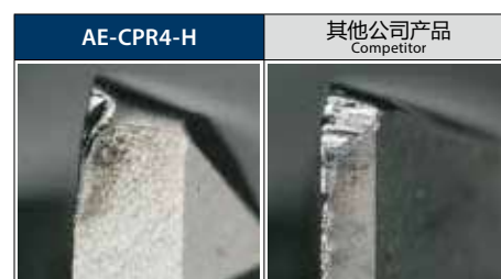
加工80.2m (型腔14个) 后的刃尖磨损情况 Wear condition of outer peripheral cutting edge after milling 80.2m
